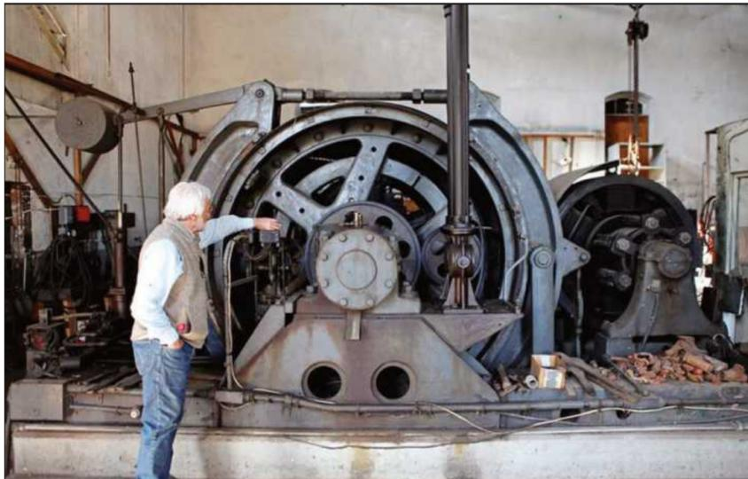
THE ORIGINAL HOIST ENGINE that lifted copper from the depths of the Keweenaw Peninsula for years after the Champion Mine was closed in Painesdale in 1967. It was later used to pump water for municipal use by Adams Twp. Newer water pumps eventually replaced it. Photo credit: Visit Keweenaw
