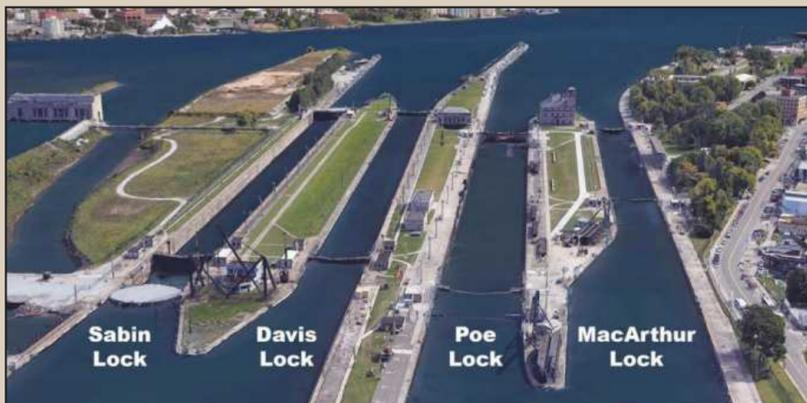
A PRE-CONSTRUCTION aerial image of the Soo Locks. The Army Corps of Engineers is building a second Poe-sized lock to provide much-needed resiliency for ship movement throughout the Great Lakes. The new lock is being built on the existing Sabin and Davis lock sites.
